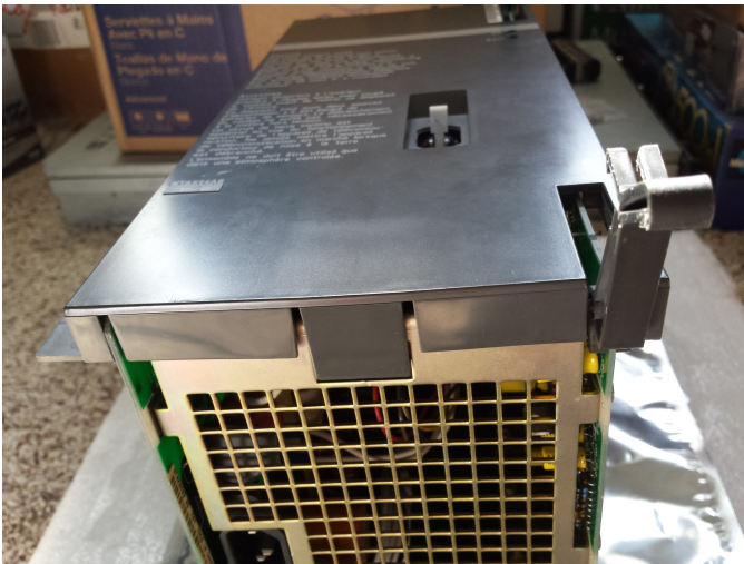
Fig. 2: Retaining clip to remove the front of the power supply
