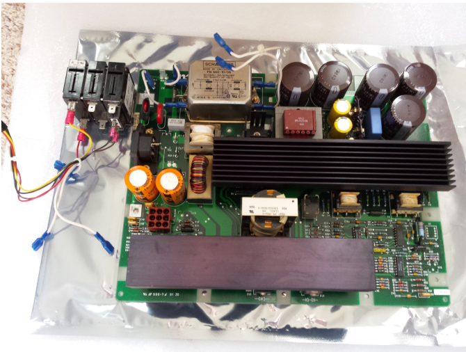
Fig. 11: Breaker assembly separated from AC board
